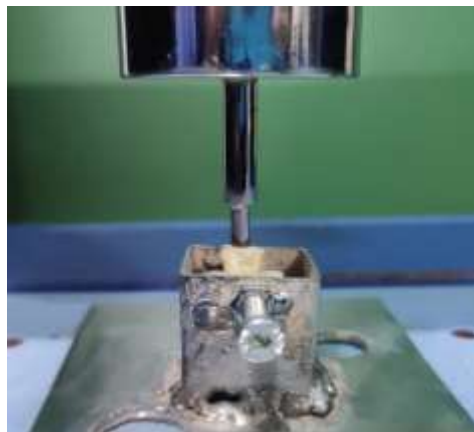
Figure 1: Sample mounted in self-cure acrylic resin subjected to universal testing machine
