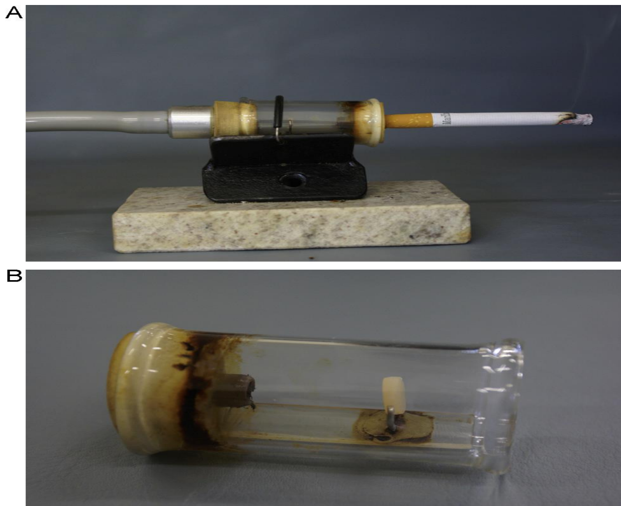
Fig. 1 – (A) Smoking equipment used in the study. (B) Specimen put into the chamber using a supporting device.
