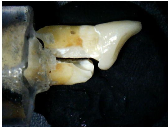
"Figure (13): Representative microscopic image of failure mode C (X30)"
