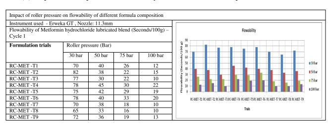
There is significant increase in the solid fraction with increase in the roller pressure irrespective of nature of diluents and presence or absence of binder. This helps in increase densification and hence help in enhancing flowability.
