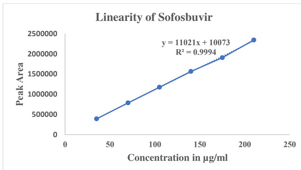
Figure2: Calibration curve of Sofosbuvir in the range 35 to 210 µg/ml.
