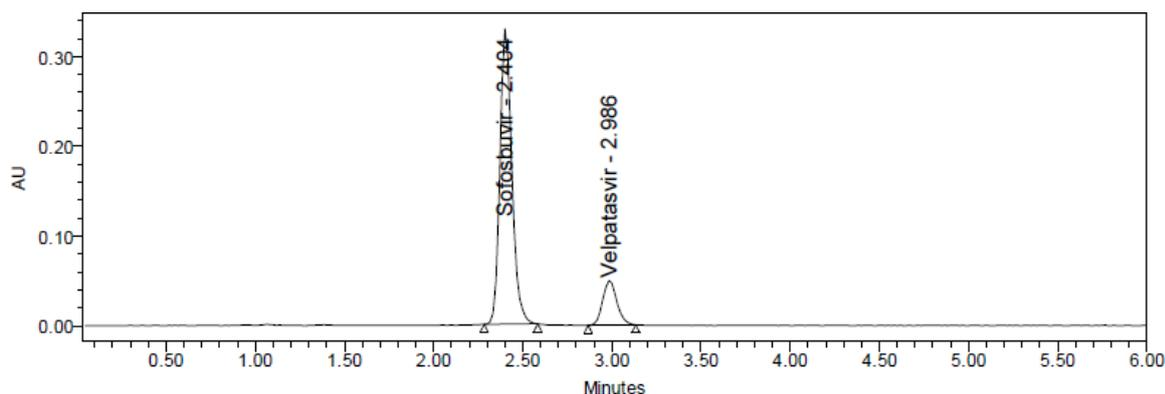
Figure1: chromatogram of Sofosbuvir and Velpatasvir in optimized chromatographic conditions
