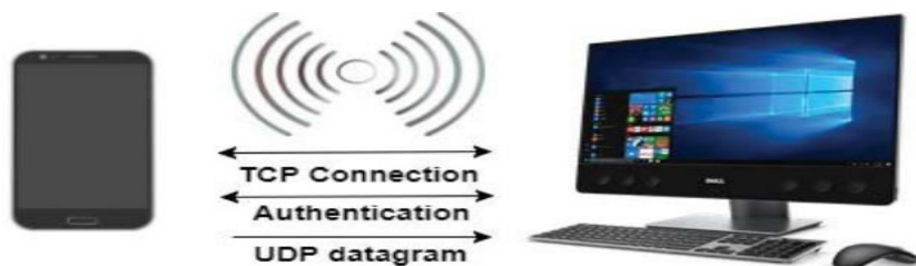
Figure 2: Data flow from smartphone to the laptop.
