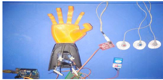
Fig. 9: Sample Working Mechanism of the Prosthetic Hand
